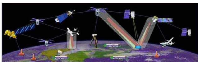
Figure 1 - Using a Sensor Web as a set of interlinked sensor platforms to perform collaborative observations. Graphic Credit: NASA/GSFC: 2000 Survey of Distributed Spacecraft Technologies and Architectures for NASA’s Earth Science Enterprise in the 2010-2025
